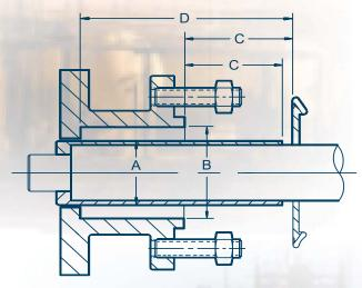
To provide superior seal performance, the Model 510 seal configuration is pump specific. The dimensions shown below are minimum equipment requirements and are for reference only.
